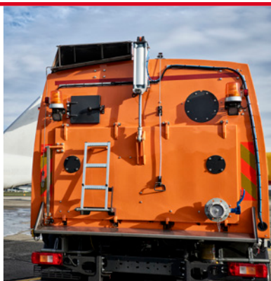
Functionality everywhere Rear door for emptying and maintenance, safety beacons, and a practical ladder and hose coupling on the back.
