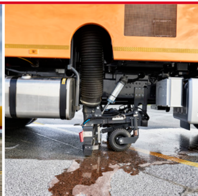
Wide suction Effective liquid recovery with a highly efficient wide suction. Useful in airports to remove glycol from the stand.
