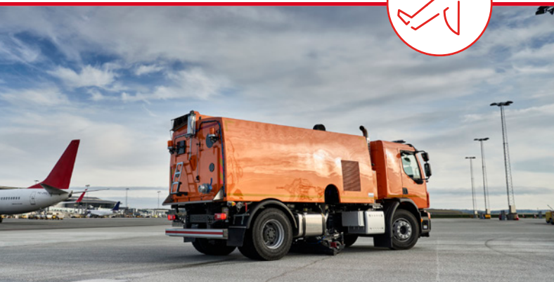
Bucher XPowa aero Powerful sweep gear and water system configured for stand cleaning and glycol recovery.
