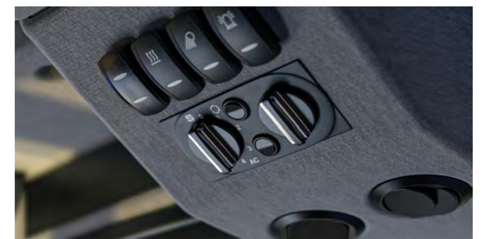
Instrumentation All switches are also within easy reach on the overhead console with the air-con controls.
